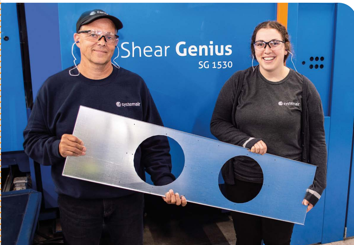
Ron Gallant , fabrication/maintenance manager, and Sylvie LeBlanc , production manager, inspecting a part produced through Shear Genius punch/shear combination.
